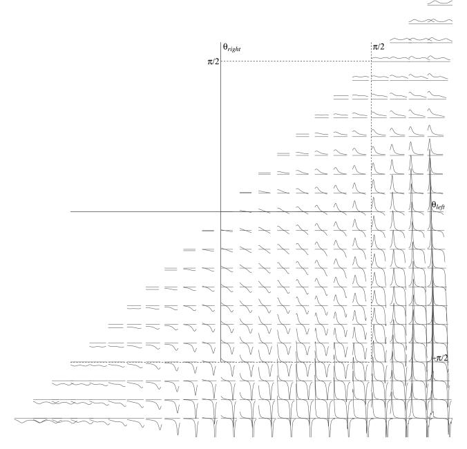
Figure 1.9: Curvature plot of Hobby spline over its parameter space.
