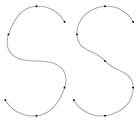
Figure 1.10: Circle spline extensibility failure.
