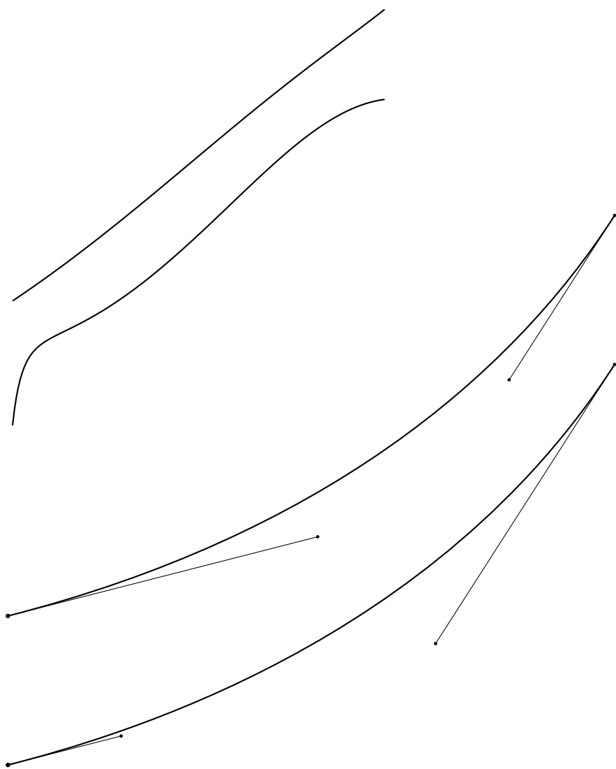
Figure 9.6. Local minima of cubic Bézier fitting, t=[0.5, 1.0] . Curvature plots are the top two graphs, the Béziers are on the bottom.
