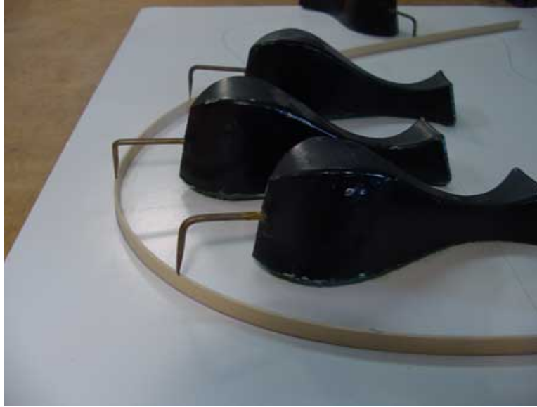
Figure 3.19. High-friction spline constraints on a real spline.
