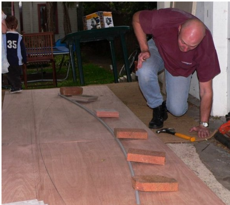
Figure 3.19: Bricks as high friction constraints on a real spline.
