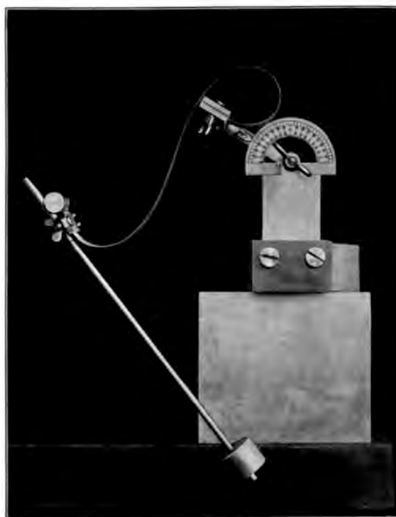
Figure 5.16: Born's experimental apparatus for measuring the elastica.
