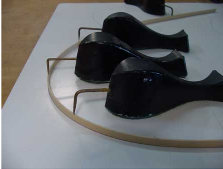
Figure 3.18: High-friction spline constraints on a real spline.
