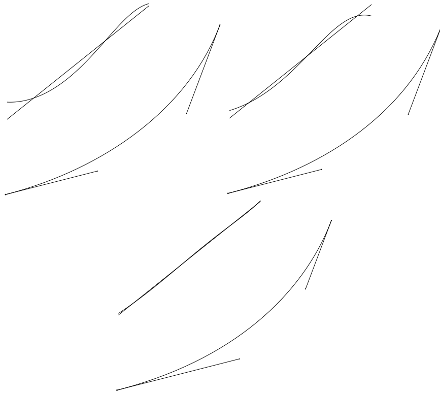
Figure 9.4. Three Bézier solutions: fast, equal arc length, and fully optimized. Curvature plot is the top graph, the Bézier is on bottom.
