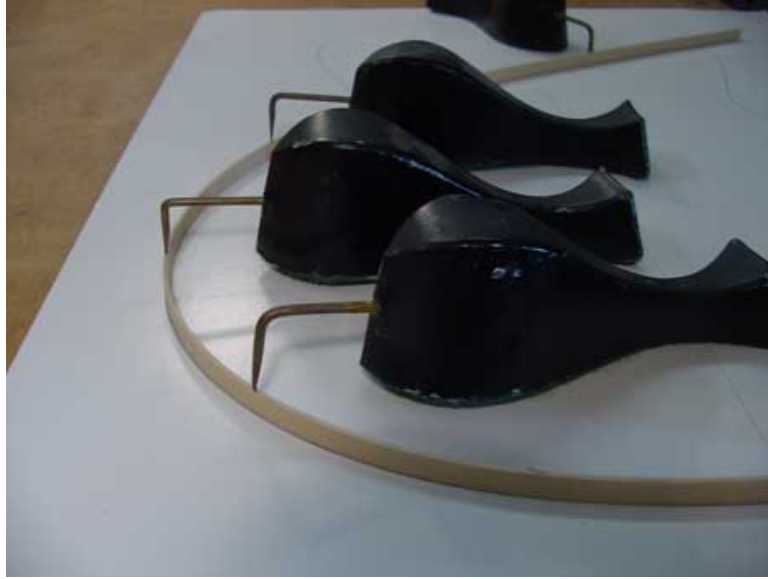
Figure 3.19. High-friction spline constraints on a real spline.
