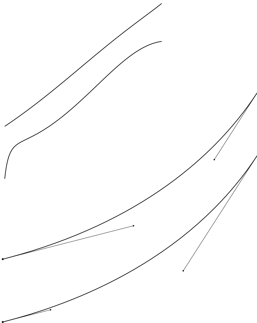
Figure 9.6. Local minima of cubic Bézier fitting, t=[0.5, 1.0] . Curvature plots are the top two graphs, the Béziers are on the bottom.
