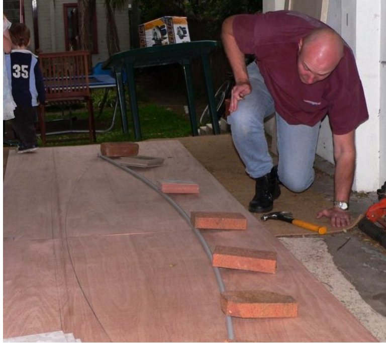
Figure 3.20. Bricks as high friction constraints on a real spline.
