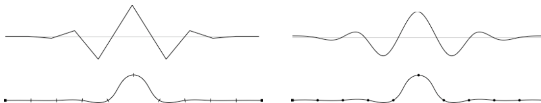
Fig. 4: Curvature behavior and resulting shapes for a G^2 -spline (left) and a G^4 -spline (right).
